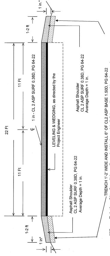
Note: Shoulder needs grass graded before resurface. This item is incidental to Pavement Bid Items. \*Where Existing Site Conditions Permit, Wedge with DGA as directed by the engineer.
